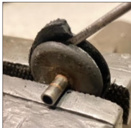
Cut, or chip out the old rubber wheel. You will find it is quite hardened and comes in pieces
