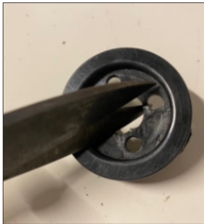
Cut new freewheel. Some come pre-cut, others do not
