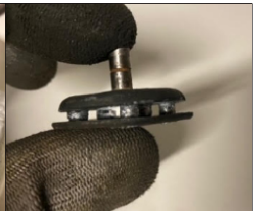
The metal rim, minus the old rubber, The new just stretches on, lining up holes with rivets
